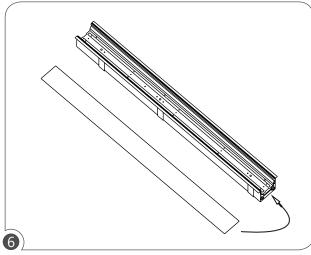
Reinstall LED module plate and lens.
