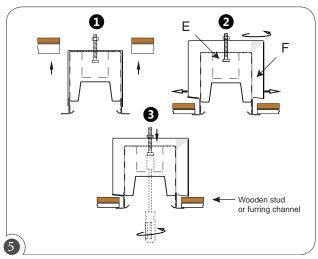
Push safety bracket screw(E) up to Rotate safety brackets(F) once bracket is correctly align tighten screw to lock fixture in to drywall ceiling.
