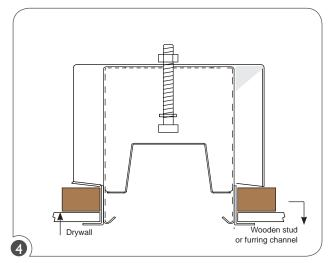
Align fixture to pre-cut hole on drywall and insert fixture.
