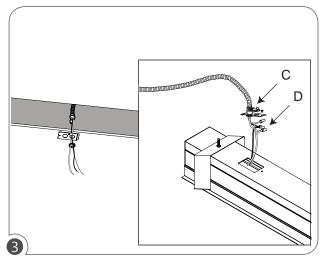
Install BX cable connector(C) to access plate(D). Wire BX cable wires to Fixture wires.
